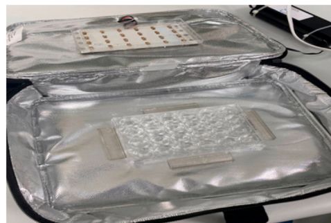
Figure 2. Interior of Clean Bag II (O2 Led) with 24-well plate arrangement.
