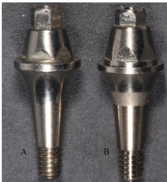
Fig. 1. Photographs of the abutments used in this study. (A) Control group: conventional intermediate abutment with a smooth surface. (B) Test group: intermediate abutment with a 1.5-mm collar surface-treated with TiO 2 .
