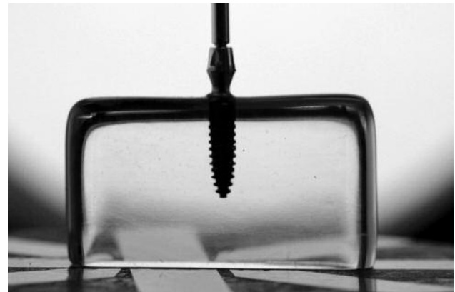
Figure 8. Photoelastic analysis of the model without residual stresses
