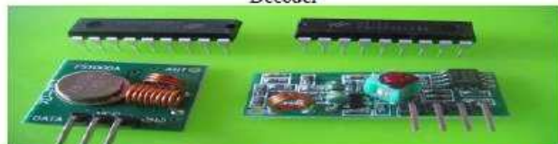
Figura 1 – Módulo Rf 433,92, Transmissor, Receptor, Encoder e Decoder
