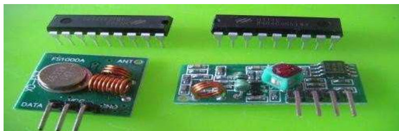
Figura 3: Módulo Rf 433,92, Transmissor, Receptor, Encoder e Decoder
