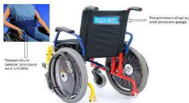
Fig.6. Illustration of an Automated Wheelchair with Radio Frequency control (ControlHelp 1.1) coupled to it, an Arduino display for temperature and pressure.
