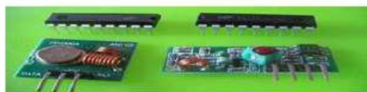
Fig.1. Module RF 433.92, Transmitter, Receiver, Encoder and Decoder.
