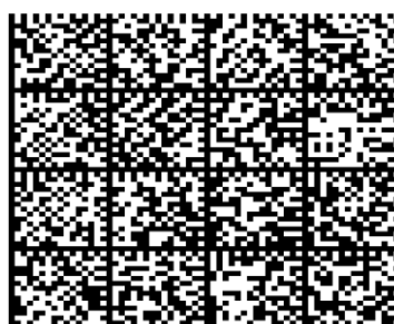
Fig. 1. Example of a two dimension code (2D), type DATAMATRIX.
