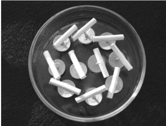
Figure 1. Experimental model. Glass Petri dish with pellets inserted in each pushpin
