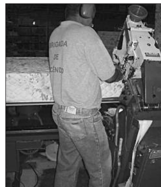
Figure 6. Positioning of sewing – Machine without platform
