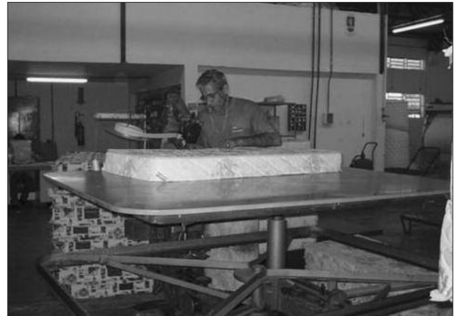
Figure 4. Sewing positioning: table with platform
