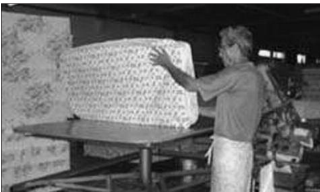
Figure 5. Movement to manipulate the mattress: table with platform
